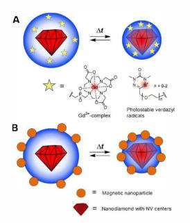
Fig. 14: Structure of hybrid temperature nanosensors based on readout of changes in magnetically active thermoresponsive polymer coating. A) Crosslinked shell loaded with spin labels, B) Magnetic nanoparticles installed on surface of thermoresponsive polymer.
