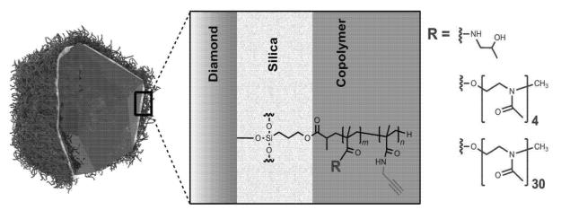
Fig. 13: Poly[N-(2-hydroxypropyl) methacrylamide] and two brush-like poly(2-methyl-2-oxazoline)-based co-polymers grafted from a nanodiamond particle. The chains contain also alkyne groups for rapid and highly bioorthogonal "click" conjugation chemistry suitable for aqueous environments.
