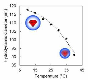
Fig. 15: Nanodiamonds coated with a thermoresponsible polymer show monotonous decrease with increasing temperature (unpublished results).
