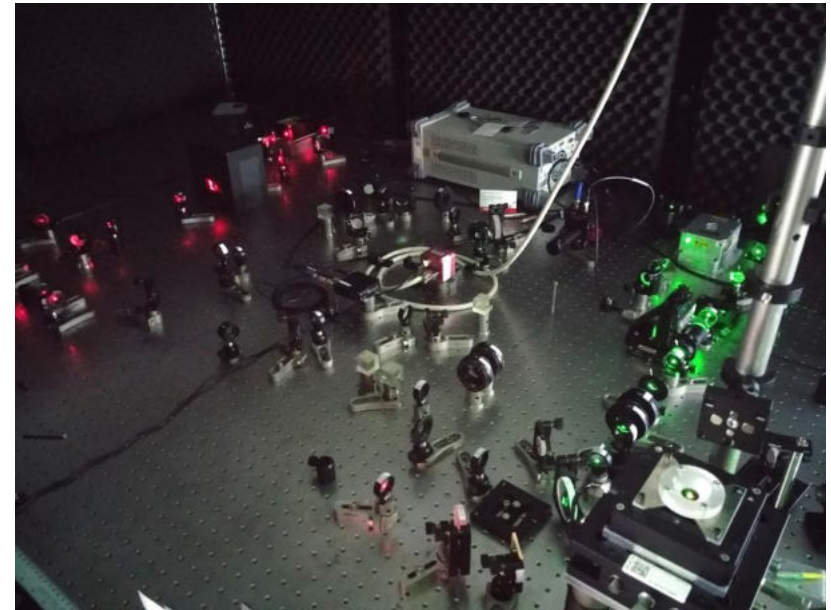
Fig. Experiment for ultrasensitive monitoring of a single-protein anisotropy.
