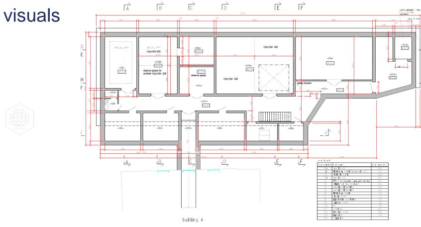
study of Cryo electron microscope installation in the IOCB complex floor plane of 2. underground
