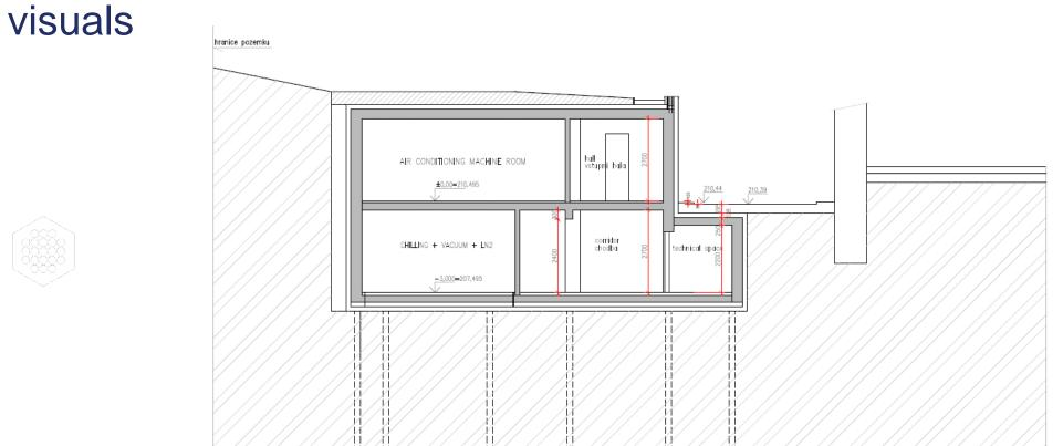
study of Cryo electron microscope installation in the IOCB complex section FF
