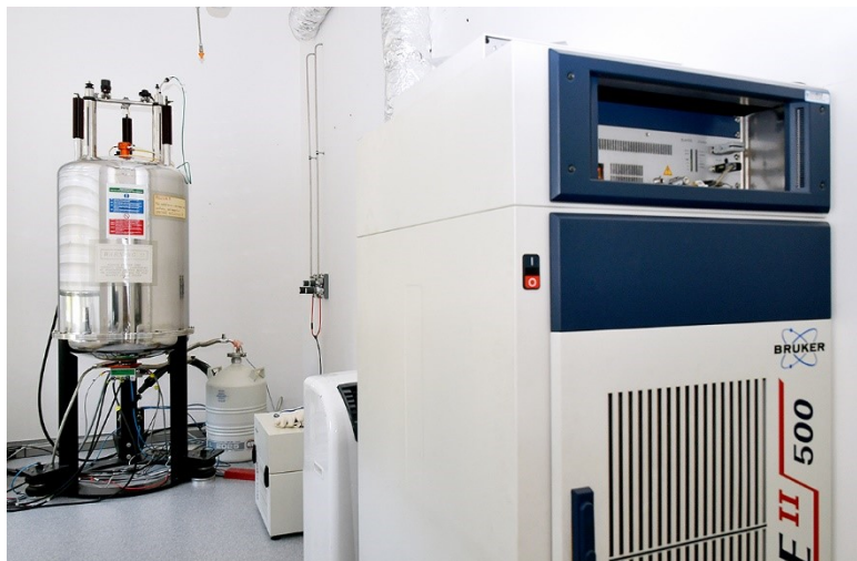
Bruker Avance II 500 MHz spectrometer 3.2 mm MAS probe
