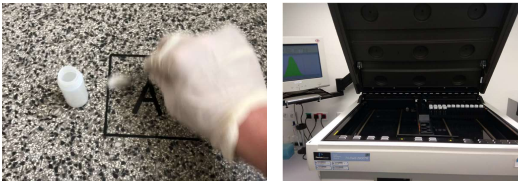
Figure 5. Survey monitoring performed by swipes with cotton measured by LSC technique
