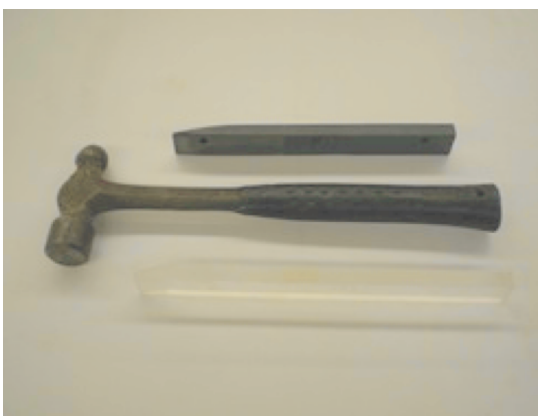
Figure 9 (right). Blunt defrosting tools are very important, and can be made from soft Polyvinyl Chloride (PVC) or Polypropylene (PP) plastic and used with gentle hammering if needed.
